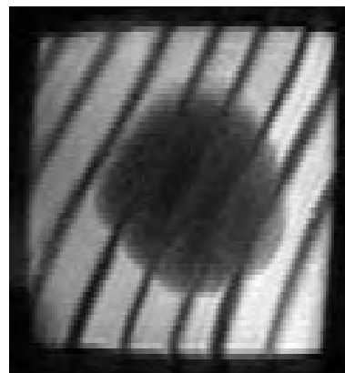
Figure 6. Image of a pine bar of a square cross section of (1.7 \text{ cm})^2 and 5 cm in height. The bar was initially frozen and was melting during the MRI experiments.
